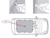
3. Move into the vehicle as shown, install and adjust the buckle. Press the center logo to complete the installation.
